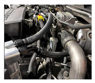
**Step 7:** *CUT* one section of hose to 17" (precut) and connect it from the outlet side of the catch can to the intake air horn. Cut the other section of hose to 14" and connect to the inlet side of the catch can and the other side to the CCV block (180-degree fitting)
