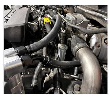
Step 8: Using the worm drive clamps SECURE the hose at all connection points
