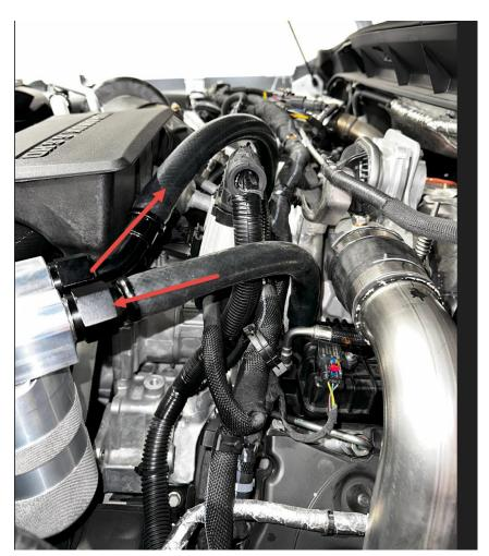
**Step 4:** Using the supplied worm drive clamps fully tighten on all 4 connection points
