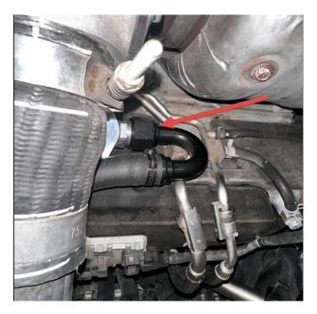
**Step 6: INSTALL** the fittings on the catch can as shown below and tighten. The straight fitting (or 45-degree fitting your choosing) goes to the intake air horn on the **OUTLET** side of the catch can. The 45-degree fitting goes to the 180-degree fitting on the CCV block.
