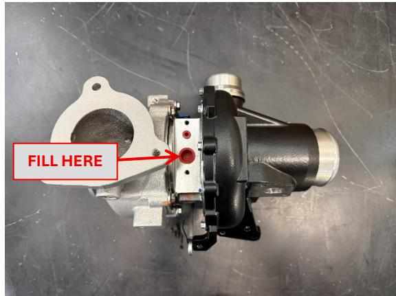
2. Using clean engine oil, fill the inlet to the top of the threads
