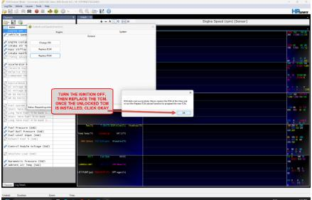
6. With the Unlocked TCM installed, select Replace TCM again
