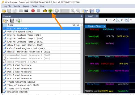
3. Select the System Tab, then Replace TCM (STOCK TCM MUST BE INSTALLED)
