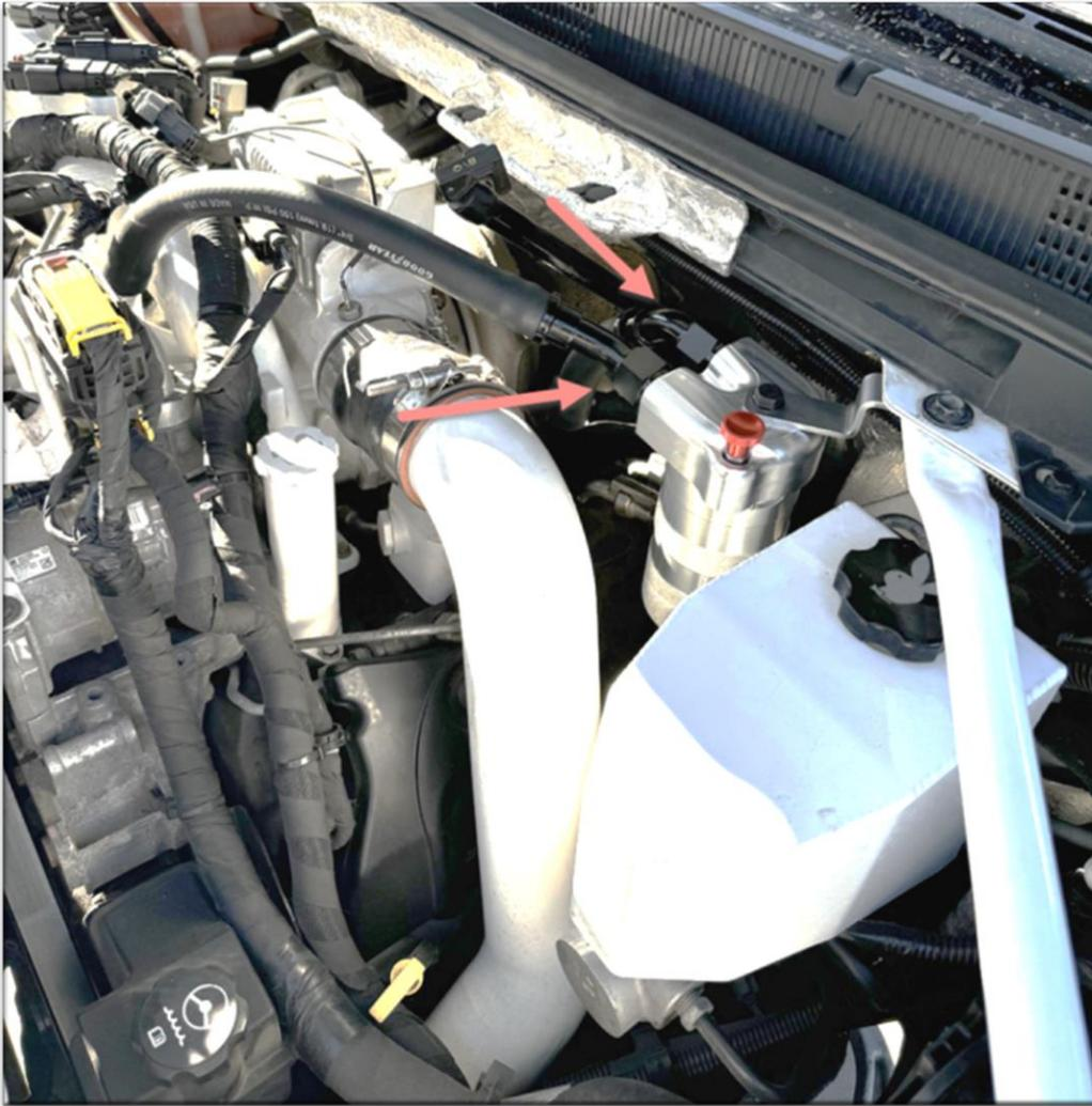
**Step 5: INSTALL** the supplied 90-degree fitting on the back (firewall side) of the CCV block.
