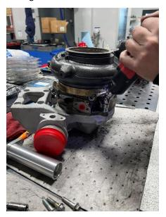
• With the intake housing now removed, place a 19mm socket in a vice or rig a stand to allow the turbine nut to sit in the socket vertically and stationary.
